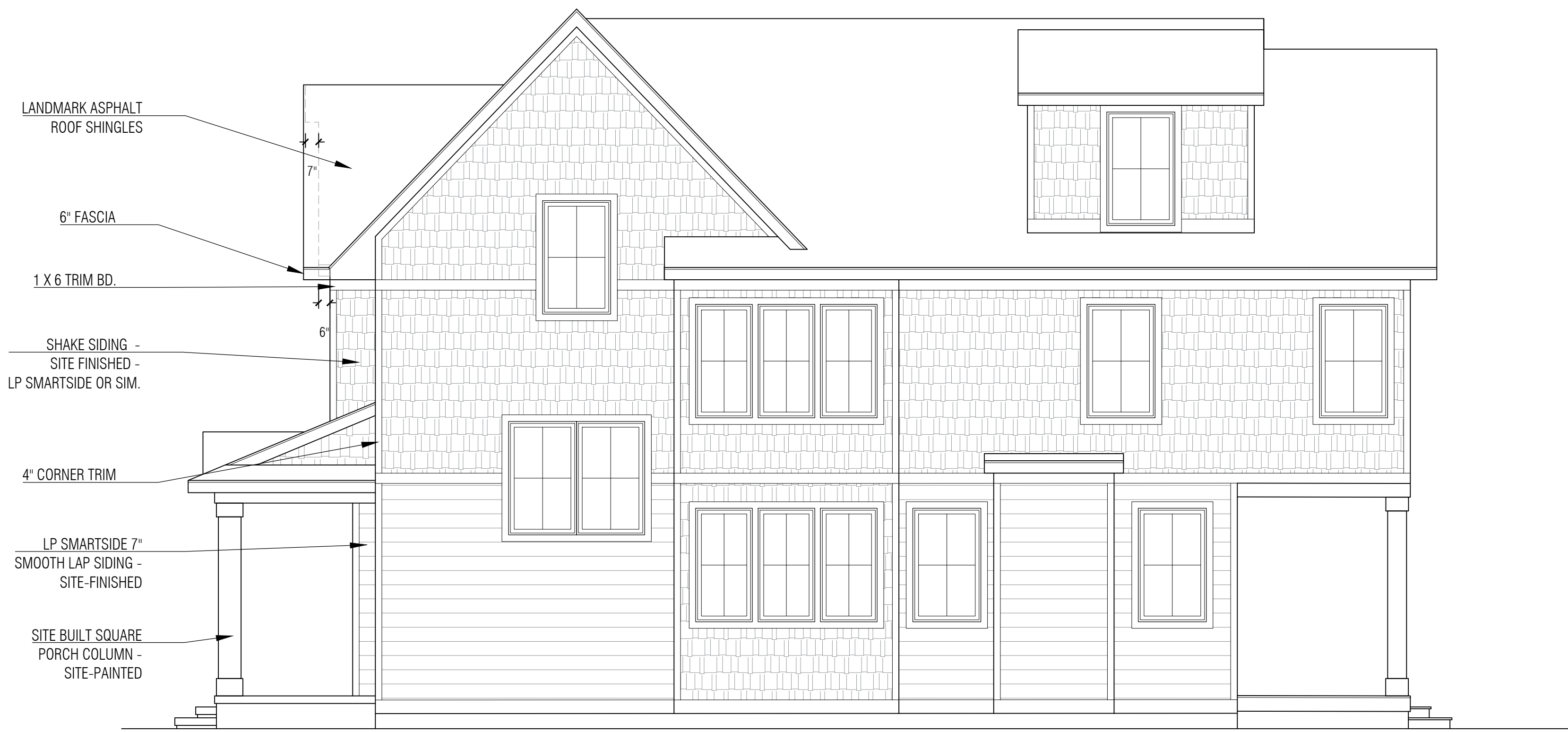
PROPOSED RIGHT ELEVATION SCALE: 1/4" = 1'-0"
